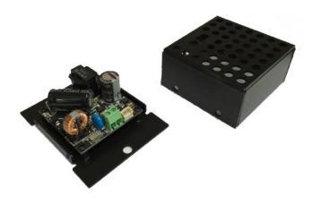
The **Remote Alert** inADAC24PM power module enables the use of the 12VDC in30 ATM camera on 24VAC powered systems. This allows the installer to use both 24VAC and 12VDC powered cameras on a common 24VAC power infrastructure. The power module is mounted to a back plate and has a removable shield to help prevent EMI/RFI issues within the ATM. This unit ships with a 36" power/video cable which allows mounting of the power module in back of the ATM.
